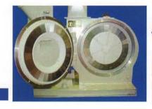
PALLMANN Pulverizing Installation Type PKM for economical pulverizing of PVC pipe granules
