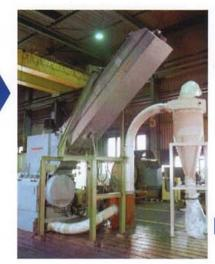
PALLMANN Pipe Crusher for size reduction of PVC pipes, with tilting funnel for feeding from the top.
