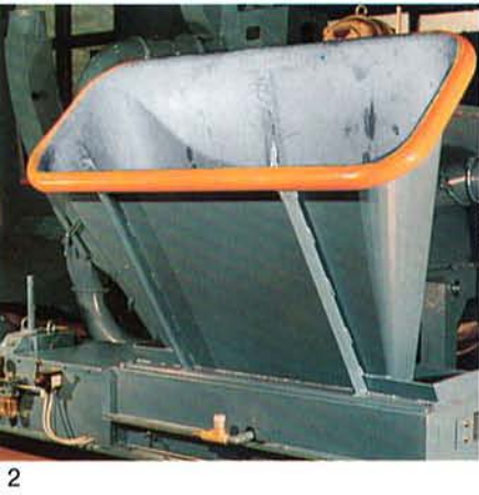
Fig. 1: Knife Mill system with model PS 8-15 for the direct recycling of polyester film waste.
