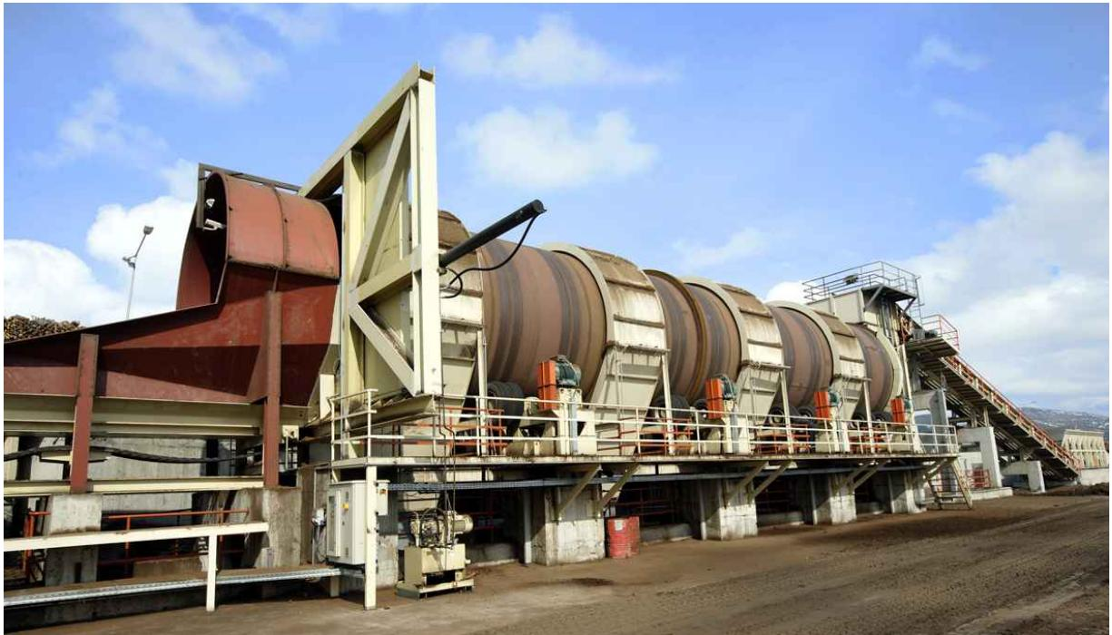
Logs have to be debarked in an economical and reliably manner to fulfil the requirements of modern product lines. Excellent debarking performance is specially imposed by the MDF- OSB and wood pellet industry.
